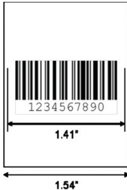
Figure 7 – 10 digit Code 128 bar code on Nokia N95 display
