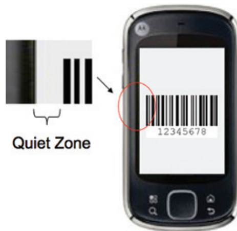
Figure 3 - Bar code plus quiet zone
