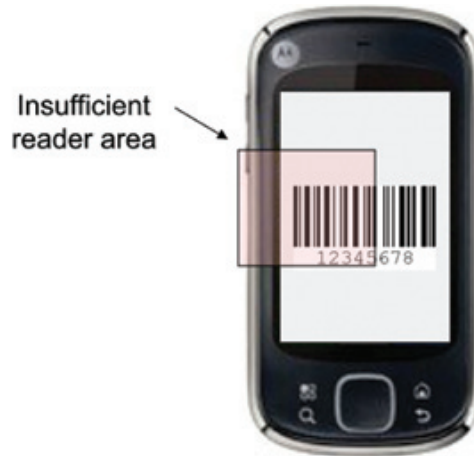
Figure 5 - Insufficient field of view
